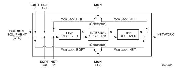
Figure 4-2. Test Jack Block Diagram
